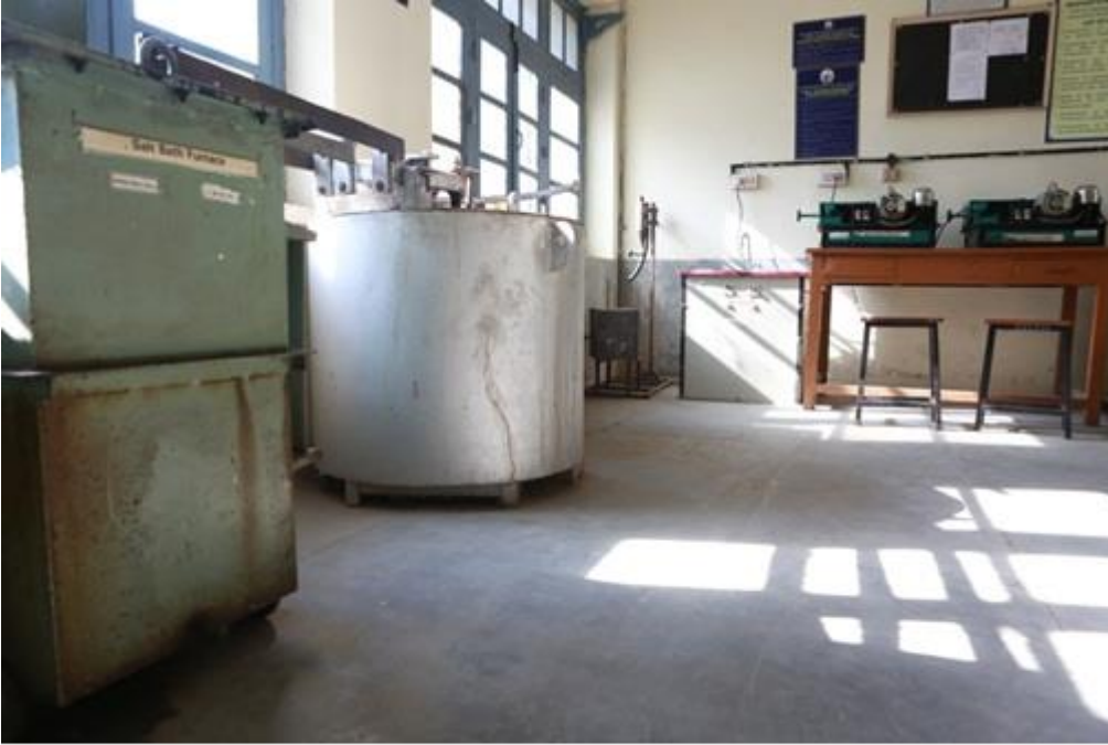
Figure 3. Salt Bath Furnace
