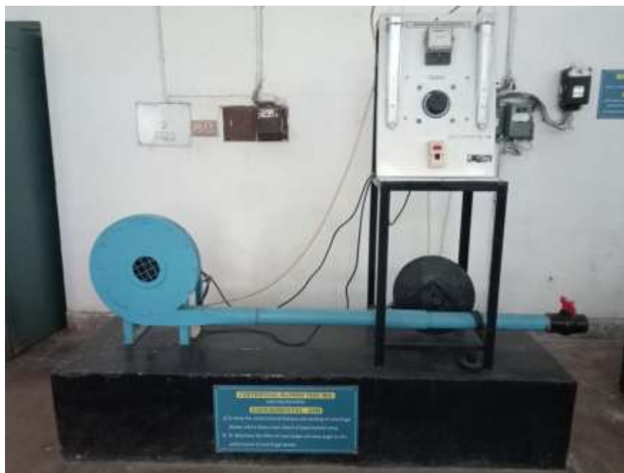
Fig.6: Centrifugal Blower Test Rig
