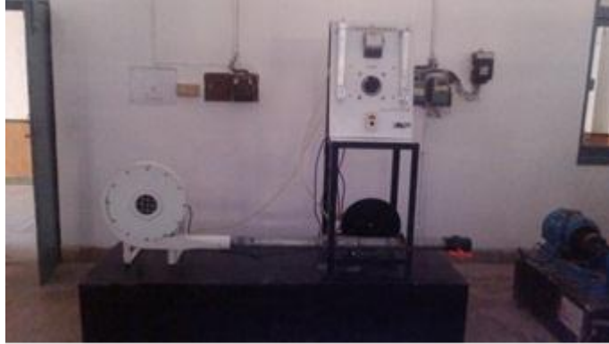
Figure 6: Centrifugal Blower Test Rig
