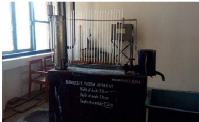
Figure 2: Bernoulli's Theorem Apparatus
