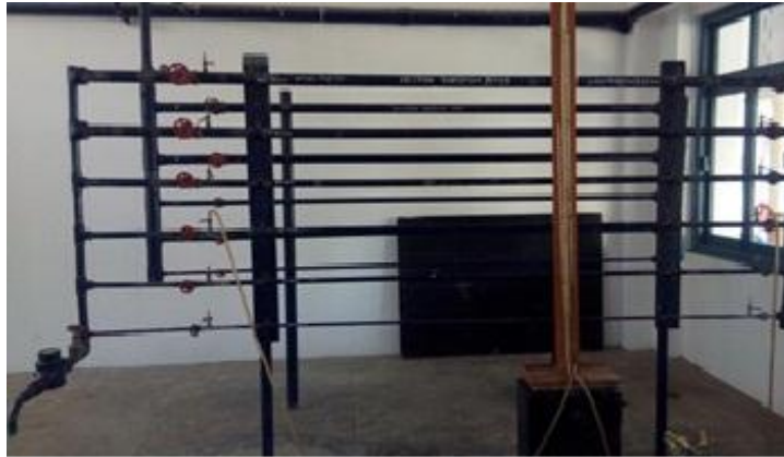
Figure 4: Friction Through Pipe Set Up
