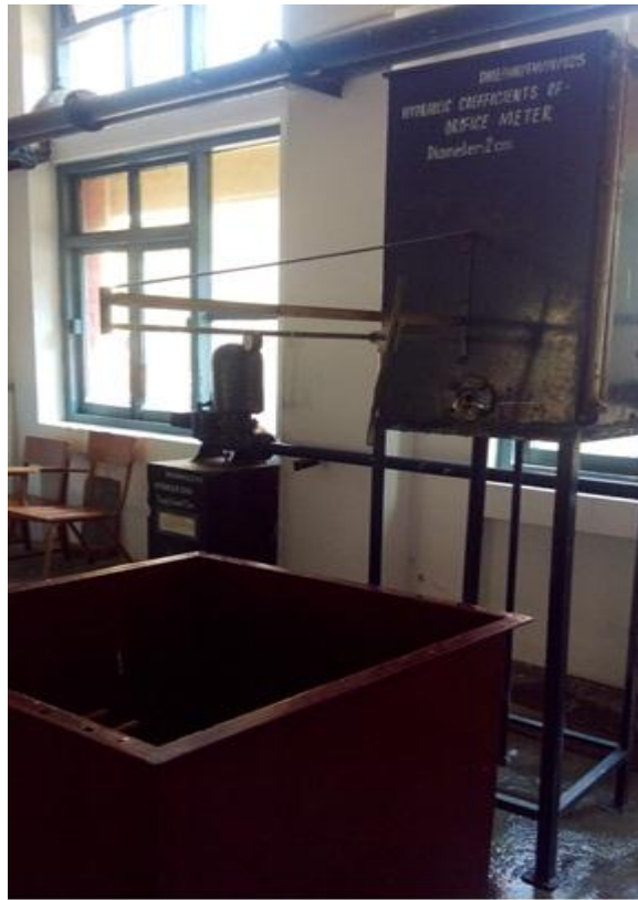
Figure 6: Hydraulic Coefficient of Orifice Plate
